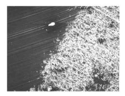
FIGURE 7(A) LEADING EDGE OF PLASTICALLY WORKED AREA OF AL FILM AFTER 3 MINUTES OF POLISHING CAF\_2 WITH 45  $\mu m$  DIA., 28 CM/S, 1 G/MM², 20KV, 102X.
