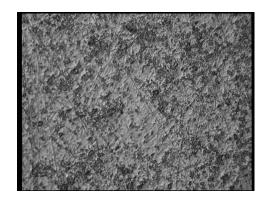
FIGURE 4(A) AU-PD COATED SILICON SURFACE AFTER POLISHING FOR 5 MINUTES WITH 25  $\mu$ m DIAMOND AQUEOUS SLURRY AT 35 RPM (W/OSCILL.), 1 G/MM <sup>2</sup>, 400X.
