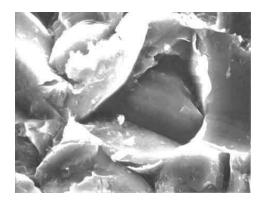
FIGURE 11(B) PARTIALLY HIDDEN EMBEDDED DIAMOND IN AL FILM AFTER 1 MINUTE OF POLISHING CAF\_2 WITH 25  $\mu m$  DIA., 28 CM/S, 1 G/MM², 20KV, 5.1KX.
