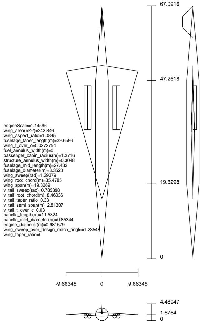
Figure 2: Supersonic transport aircraft designed by our system (dimensions in meters)
