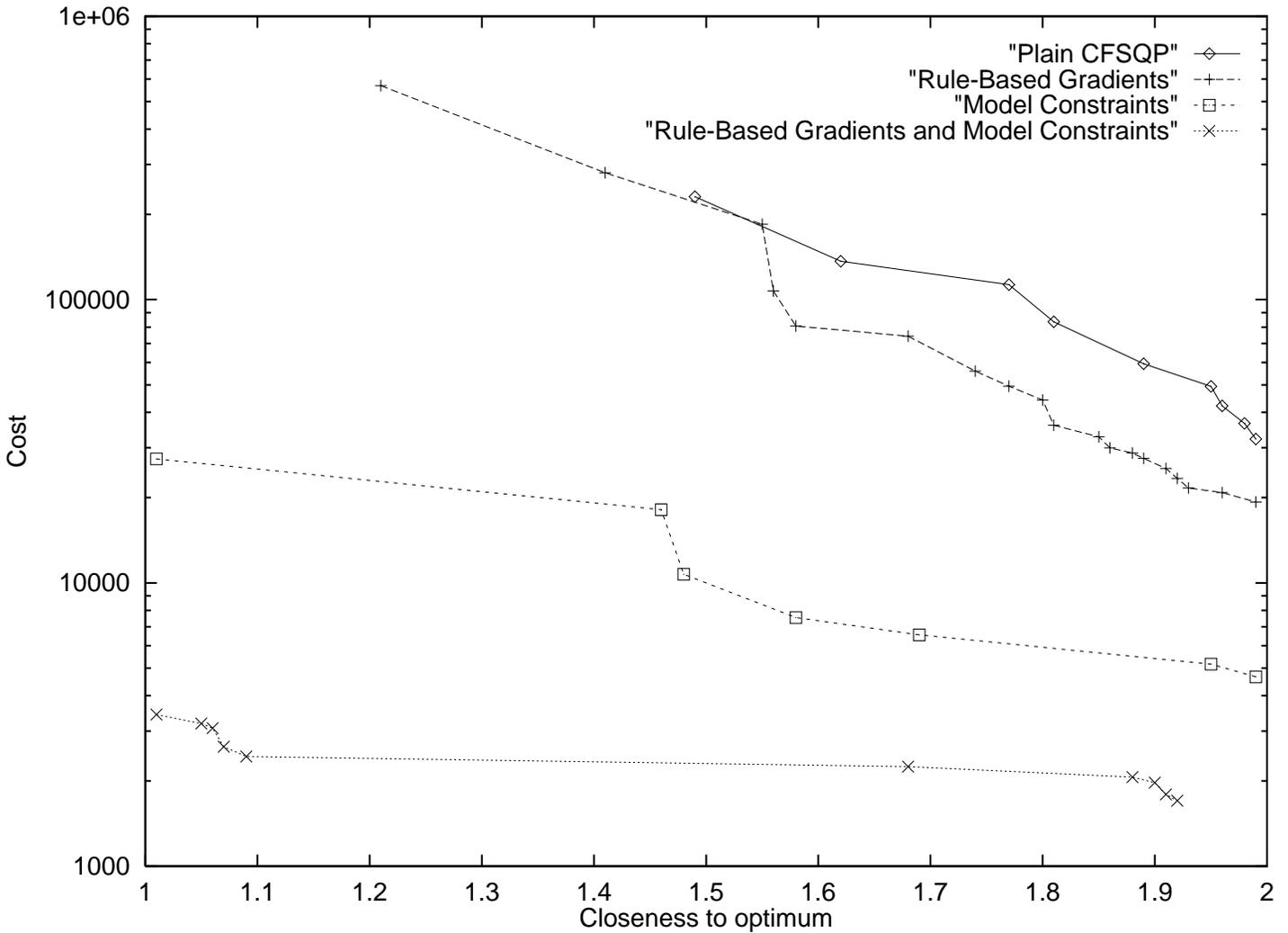
Figure 4: Performance of the various strategies. Optimization performance increases as one moves down (lower cost) and to the left (closer to the apparent global optimum). The cost shown is the estimated number of simulations needed to have a 99% chance of getting within the specified fraction of the optimum.
