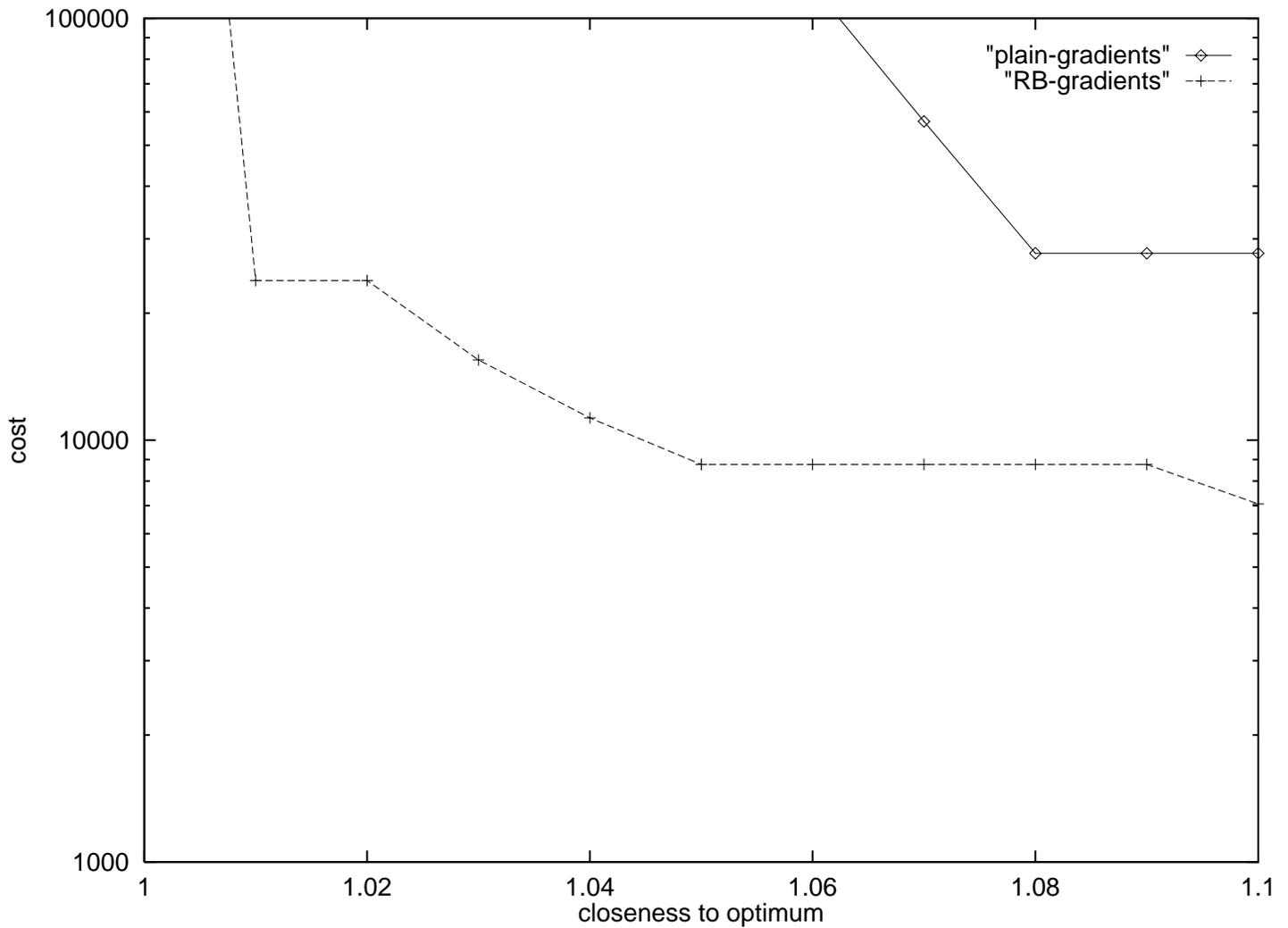
Figure 6: Performance of rule-based gradients for the missile inlet domain. Optimization performance increases as one moves down (lower cost) and to the left (closer to optimum). The cost shown is the estimated number of simulations needed to have a 99% chance of getting within the specified fraction of the optimum.
