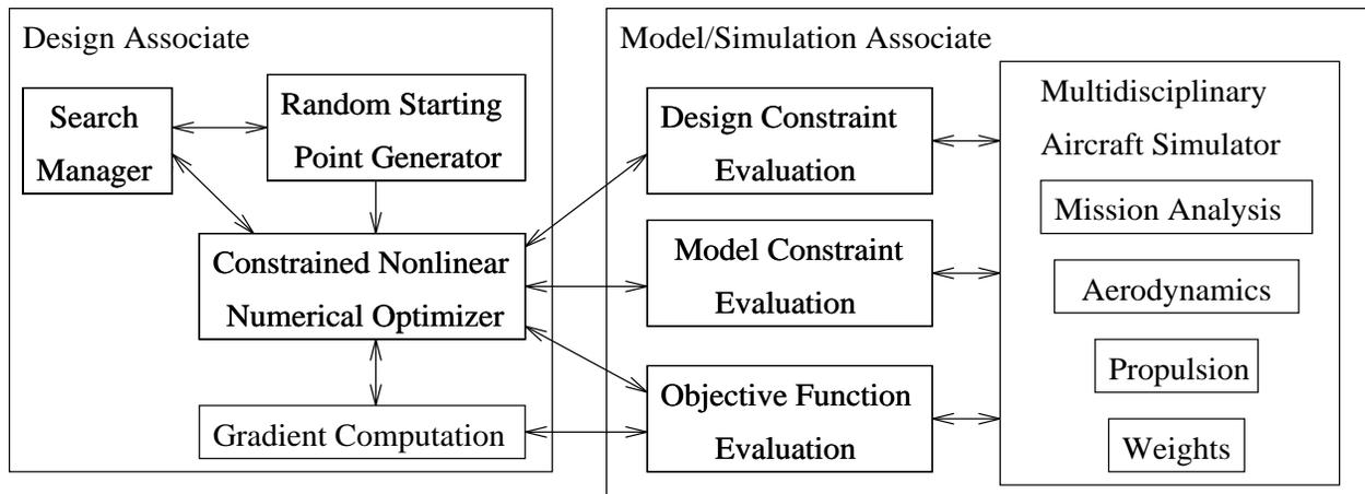
Figure 3: Automated design system block diagram
