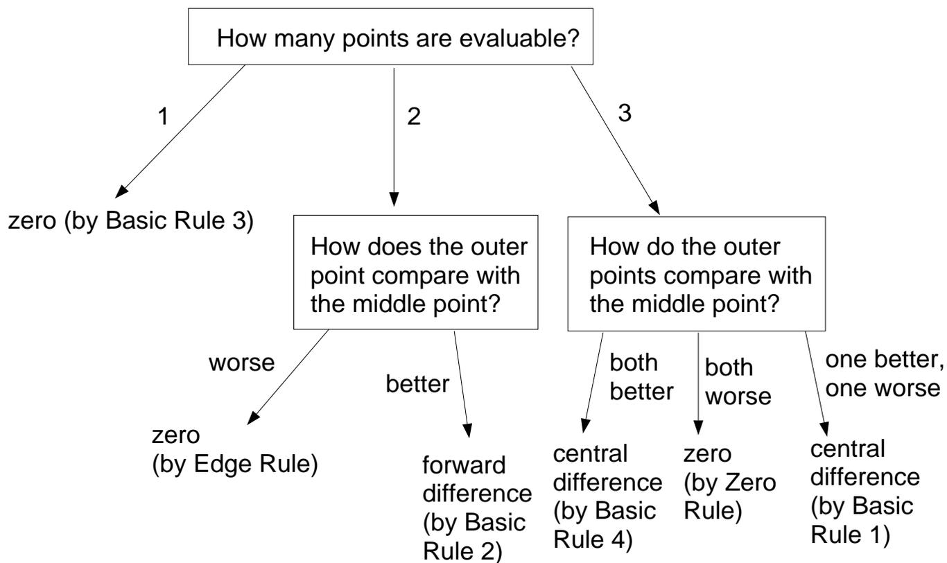
Figure 1: Flowchart of the rules used to determine how to compute a partial derivative from three points.
