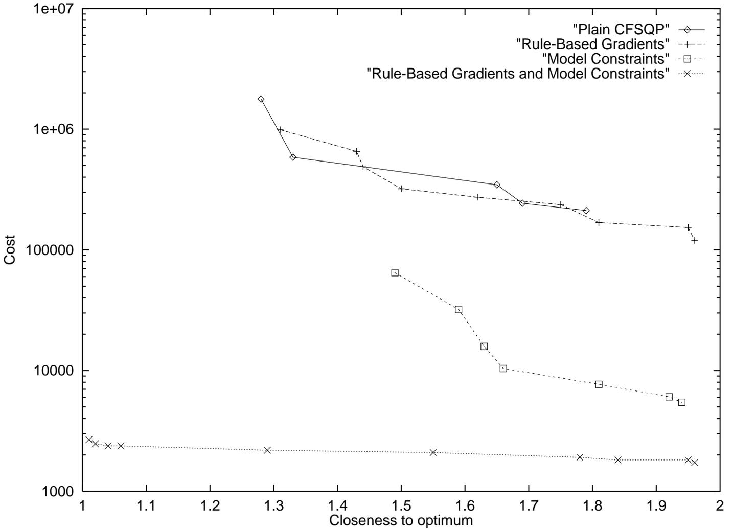
Figure 5: Performance of the various strategies for a different mission. Optimization performance increases as one moves down (lower cost) and to the left (closer to optimum). The cost shown is the estimated number of simulations needed to have a 99% chance of getting within the specified fraction of the optimum.
