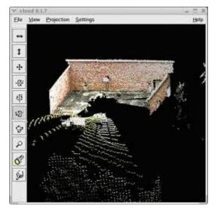
Figure 2 Data from a scan of orthogonal walls using the Riegl ladar.
