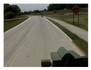
Figure 1 The first frame of a sequence. The user has drawn the features to be tracked.
