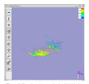
Figure 8 The sub-region seen by the GDRS ladar, taken from the same position. Elevation is again represented by color.
