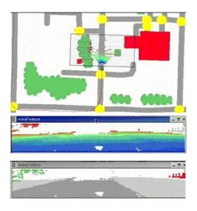
Figure 9 Top A view of the path of the NIST HMMWV traversing the NIST grounds. The features are derived from the ground truth indexed by vehicle position. The rectangle represents the field of view of the GDRS ladar. Middle. A GDRS ladar image taken from the HMMWV. Bottom. Predicted image from ground truth. Each pixel contains a label predicting the identity of the corresponding location in the ladar image.
