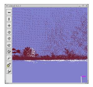
**Figure 7** The result of overlaying the GDRS ladar data on the Riegl data. The difference in measurement of the scene can clearly be seen.
