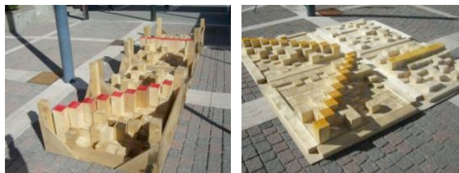
Figure 4: Step Fields provide repeatable terrain challenges.
