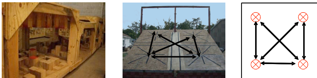
Figure 8: Mobility Tests. Left: Confined Space Cubes; Right: Inclined Plane with way point pattern
