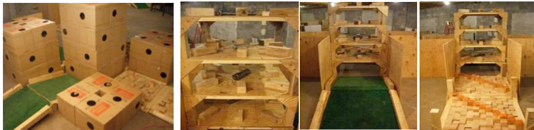
Figure 6: Left: Directed Perception Test Method; Right: three views of Grasping Dexterity Test Method. Both are shown with Pitch Ramps and Orange Step Fields
