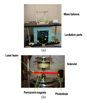
Fig. 4. (a) Proof-of-concept apparatus for a levitation mass comparison system. (b) Close-up of levitation parts in a proof-of-concept apparatus.
