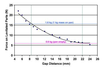
Fig. 5. Magnetic force as a function of distance between the fixed pole and the pole attached to levitated parts (gap distance).
