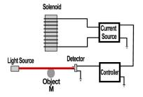
Fig. 2. Simple magnetic levitation system. A shadow detector and a feedback controller are used to suspend a ferromagnetic ball.
