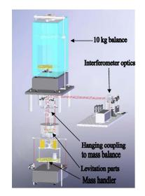
Fig. 6. Main components of the next-generation magnetic levitation mass comparison system.
