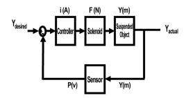
Fig. 3. Block diagram of magnetic suspension system showing the function of each element in the feedback loop.
