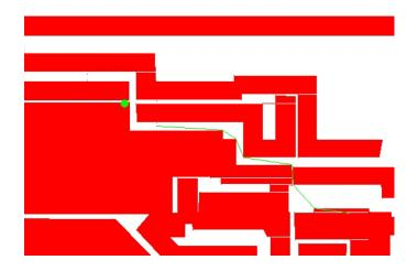
**Fig. 7.** Vector-based *a priori* map used by the *a priori* planner. The red areas are obstacle polygons and the white is free space. The computed path is shown in green, and the robot location is shown with a large green circle. The small green dots represent the planning horizon of the way-point planning system.
