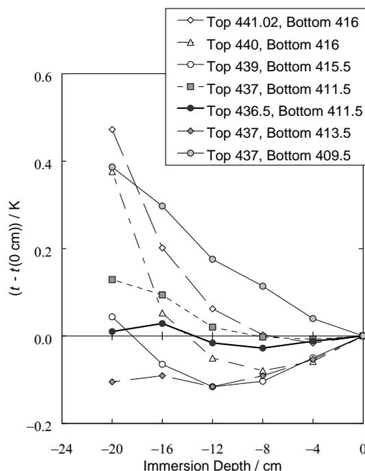
**FIGURE 2.** Immersion profiles in a silver freezing-point cell at a temperature 2 K above the freezing point, for a variety of furnace settings. For all profiles, the center zone was set at 417.5 (set point units approximately equal to  $10 \mu\text{V}$ ).
