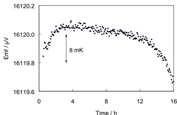
**FIGURE 4.** Freezing plateau of a silver freezing-point cell, as measured with a Au/Pt thermocouple.
