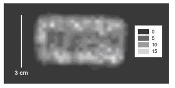
Figure 5. Pressure in kPa over the surface of the sled with the heavy weight attached. Measurements conducted on the pressure-sensitive surface (Tekscan, Inc.).
