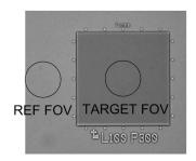
**Fig. 4** Low-magnification image of a typical grating target (target lines are unresolved), and illustration of the field of view (FOV) used for data collection. When collecting data, the field stop was reduced to restrict the area of illumination to a central area of the target (TARGET FOV) or to an area of bare silicon for the reference image (REF FOV), as shown. This image was obtained using a 10× objective, while a 100× objective was used for actual data collection.
