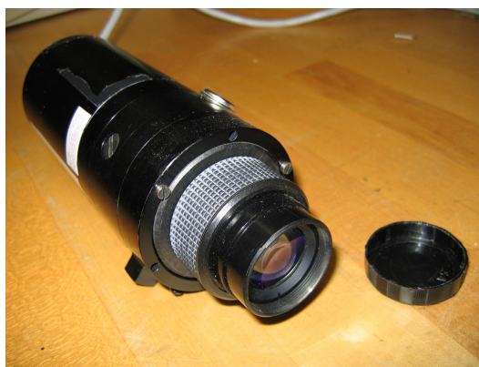
Fig. 7. Picture of the NV radiometer transfer standard with the PVS-7 input optics and the attached amplifier unit.
