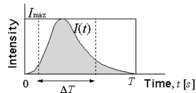
Figure 3. Schematic of the Form Factor method.
