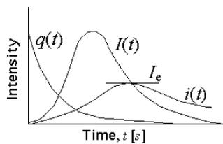
Figure 4. Schematic of the Allard method.
