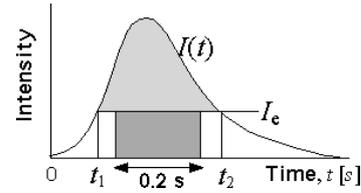
Figure 1. Graphical solution of the Blondel-Rey equation for a non-rectangular pulse.
