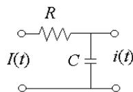
Figure 5. R-C low-pass filter circuit to achieve the convolution in Eq. (8)
