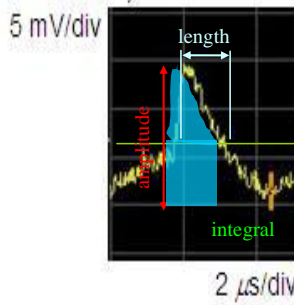
FIGURE 5. Principle of pulse characterization.
