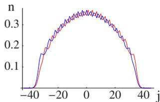
FIG. 2. (Color online) The single-atom density of species 1 (red) and 2 (blue) of a system of 90 sites, with 17 atoms of each type, with  $t/U=0.005$ ,  $U_{12}/U=0.04$ , and a trap parameter  $\Omega=10^{-5}U$ .
