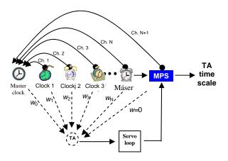
**Figure 2**. Schematic showing how the output of the micro phase stepper is held in agreement with the time scale TA.
