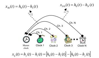
**Figure 1**. Schematic of the time difference measurement system used at CENAM, also referred to as a phase comparator. The system performs one measurement every second.
