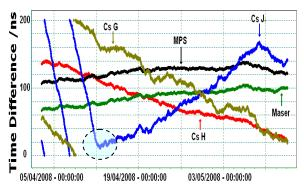
**Figure 3**. Time difference measurement of participating clocks with respect to the master clock (Cs I). The black line corresponds to the MPS output.
