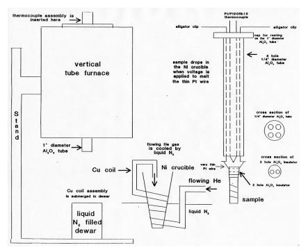
Figure 1. Schematic diagram of a quench furnace arrangement illustrating the liquid-N<sub>2</sub>cooled He quench cup and the specimen holder assembly.
