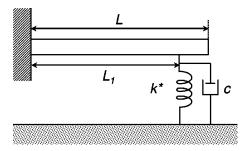
FIG. 3. Diagram of key features of AFAM model. The cantilever is clamped at one end and has a total length L. It is coupled to the surface through a spring of stiffness  $k^*$  (contact stiffness) located at a position  $L_1$  with respect to the clamped end. An optional dashpot with damping constant c is located in parallel with the spring.
