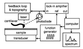
FIG. 1. Schematic of experimental AFAM apparatus.
