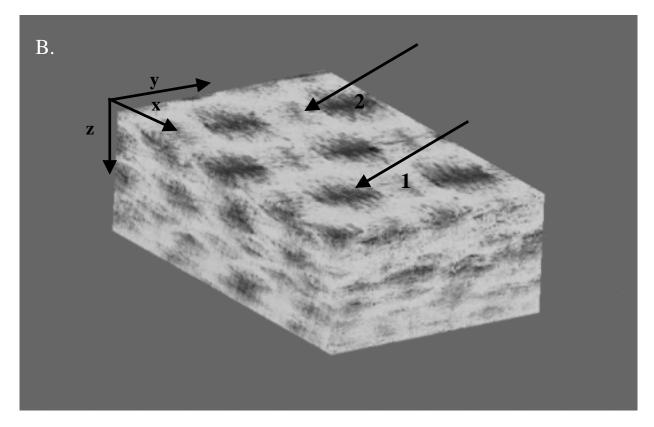
Figure 2: OCT volumetric reconstructions of an epoxy/unidirectional E-glass composite (A.) and an epoxy/ $0-90^{\circ}$  woven E-glass composite (B.).
