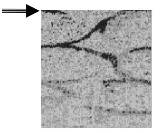
Figure 3: OCT image of impact damaged epoxy/unidirectional E-glass composite. 0  $\mu$ m from surface along the x-z plane (A.). Along the y-z plane showing placement of tows via polyester stitching (B.).
