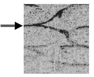
Figure 7: OCT image of impact damaged epoxy/unidirectional E-glass composite.  $652 \mu m$  from surface along the x-z plane (A.). Along the y-z plane showing placement of tows via polyester stitching (B.).
