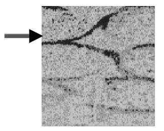
Figure 5: OCT image of impact damaged epoxy/unidirectional E-glass composite. 460  $\mu$ m from surface along the x-z plane (A.). Along the y-z plane showing placement of tows via polyester stitching (B.).
