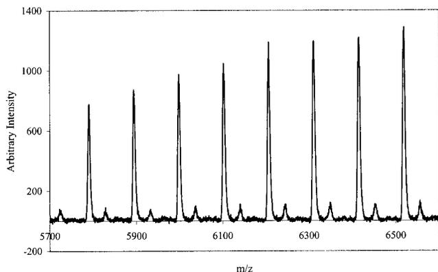
Figure 3. MALDI-TOF-MS MMD of PS expanded to show the secondary peak series.
