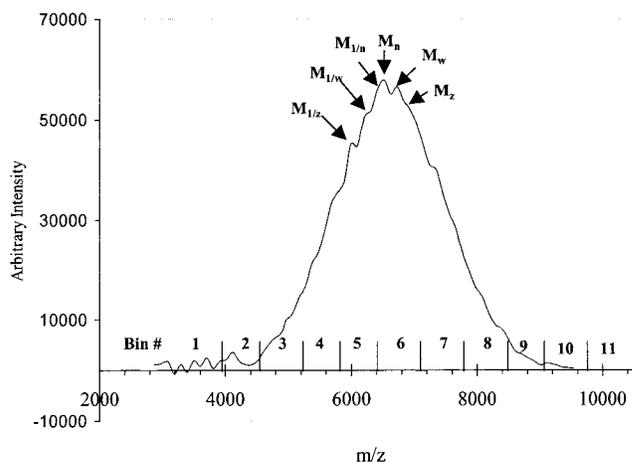
Figure 4. Moments and bins shown in relation to the integrated PS MMD. The moments represent the center of the MMD, whereas the bins represent the entire distribution.
