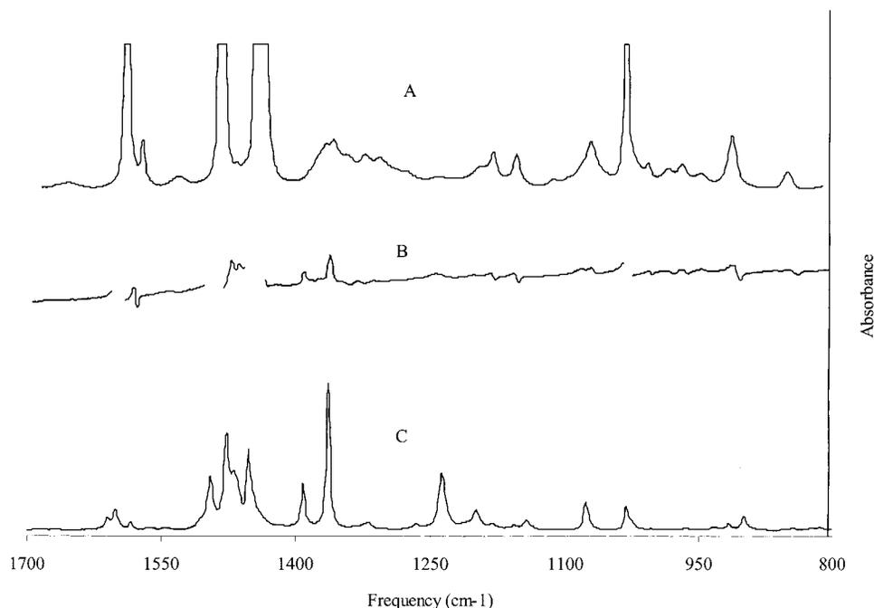
Figure 1. FT-IR spectrum of the MALDI PS (A), neopentylbenzene (C), and the difference spectrum, MALDI PS – SRM1479 (B). Peaks identifying the *tert*-butyl end groups are at 1365, 1393, and 1475  $\text{cm}^{-1}$ .
