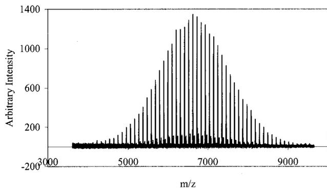
Figure 2. MALDI-TOF-MS MMD of Interlaboratory Comparison Polystyrene using the specified recipe of retinoic acid and AgTFA.
