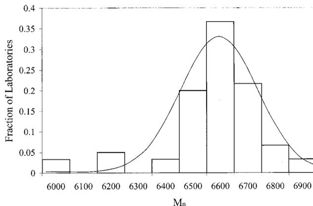
Figure 5. Histogram representing the distribution of  $M_n$ . The graphed line represents the normal distribution for the data, and the outliers are seen at 6200 and 6000 u.
