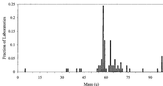
Figure 6. Distribution of the end group masses, which were calculated from the maximum peak values. The end groups, which are hydrogen and *tert*-butyl, should have a mass of 58 u.
