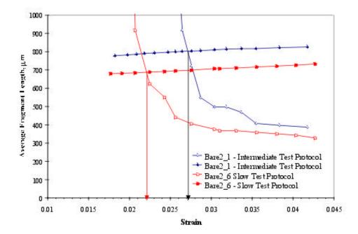
Figure 6. Graphical Determination of the 'in situ' Fiber Strength at Saturation from SFC Test Data.
