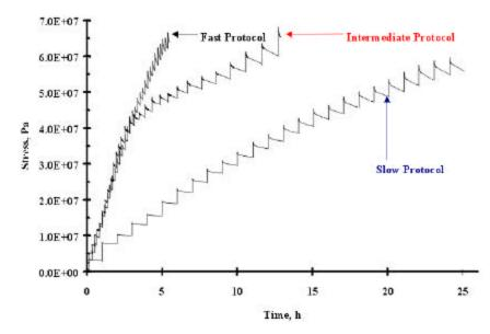
Figure 3. Stress-Time Curves for Test Protcols.
