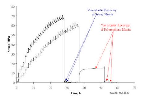
Figure 4. Matrix Recovery Profiles for Epoxy and Polyurethane Matrices.
