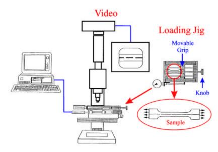
Figure 1. Schematic of Testing Apparatus.
