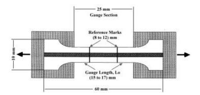
Figure 2. Typical Specimen Dimensions.
