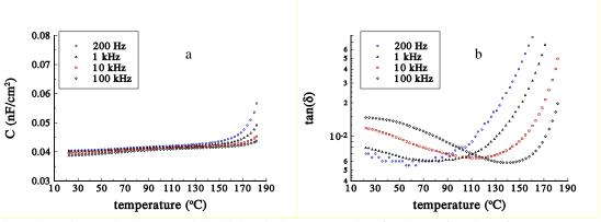
Fig.5. Capacitance density (a) and the dielectric loss tangent (b) of FR4 as a function of temperature and frequency.(TV0 / Merix, pattern B)
