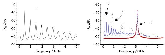
Fig.3. Measurement example using the microstrip test specimen. a) HADCO BC2000, the resonator length l=164 mm,  $\varepsilon^1 = 3.93$  at 461 MHz, b) HADCO EmCap, l=164 mm,  $\varepsilon^1 = 36.3$  at 151 MHz, c) HADCO EmCap, l=29.5 mm,  $\varepsilon^1 = 36.4$  at 842 MHz, d) HADCO EmCap l=8 mm,  $\varepsilon^1 = 35.9 \text{ at } 3.122 \text{ GHz}$
