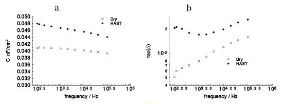
Fig.6. Capacitance density (a) and the dielectric loss tangent (b) of FR4 saturated with moisture d during HAST. (TV0 / Merix, pattern C)
