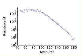
Fig.4. Insulation resistance of FR4 laminate under bias of 100V as a function of temperature
