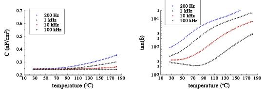
Fig.9. Capacitance density (a) and the dielectric loss tangent (b) of  $\ Hi\ K\ Kapton$  as a function of temperature and frequency. (TV0 /Raytheon-TI, pattern B)
