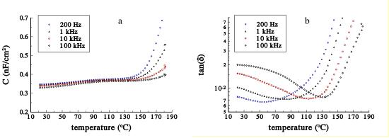
Fig.8. Capacitance density (a) and the dielectric loss tangent (b) of EmCap as a function of temperature and frequency. (TV0 / MERIX, pattern B)
