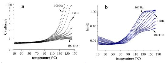
Fig.10. Capacitance density (a) and the dielectric loss tangent (b) of C-Ply as a function of temperature and frequency. (TV0/3M, pattern B)
