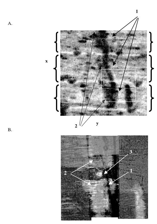
Figure 3: OCT (A.) and LSCM (B.) images 340  $\mu$ m from top surface of composite.
