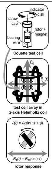
Figure 1. Multi-sample viscometer concept.
