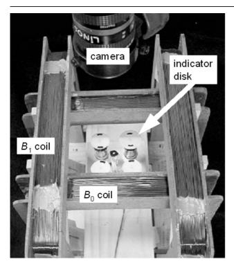
**Figure 2.** Picture of the multi-sample viscometer. The square quasi-Helmholtz coil and four test cells are shown when looking down at the instrument from an angle. The LED, used in indicating phase, is visible in the centre of the test cell array.
