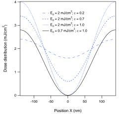
Figure 4. Exposure energy distribution along wafer plane
