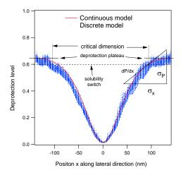
Figure 2. Deprotection profile calculated with continuous model and discrete 3-D model. All conditions are same as listed in table 1 except PEB time = 3 s. The acid loss is about 18 % within this period.
