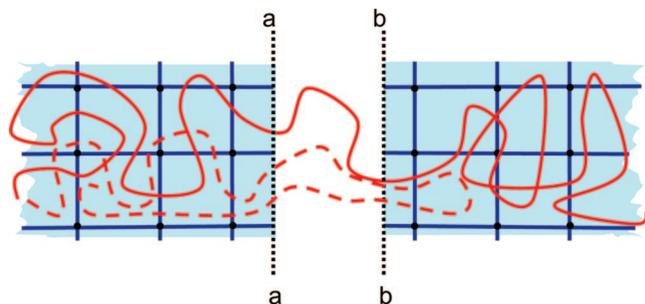
**Figure 1.** Schematic of a crack inside DN gel. The fracture surfaces *a*–*a* and *b*–*b* of the PAMPS network are bridged by PAAm chains depicted as red lines. The solid red line denotes a tie chain along which the local stress can be transferred effectively, whereas the dashed line denotes a chain that is shallowly buried on one side of a crack and hence is not an effective stress-bearing chain across the crack.
