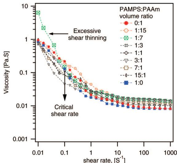
**Figure 5.** Viscosity of PAMPS/PAAM solution blends measured as a function of shear rate for various PAMPS/PAAM volume ratios. Each blend sample was prepared by mixing stock PAMPS and PAAM solutions of 0.2 mol/L concentration. An enhancement in viscosity at low shear rate is observed for 1:7 PAMPS/PAAM blend, but the viscosity rapidly decreases to a value similar to that of pure PAMPS solution beyond a critical shear rate of  $10^{-1} \text{ S}^{-1}$  as marked by the arrow.
