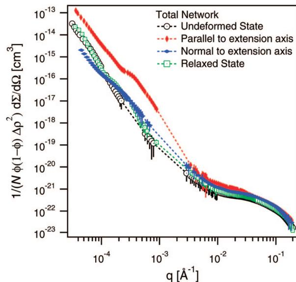
**Figure 4.** Neutron scattering from the total network measured in situ for deformed DN gels (contrast condition iii). Data parallel and normal to the elongation direction (y axis) are shown in red and blue, respectively. Results from the sample both before deformation (black) and after the deformation is relaxed (green) are also included for comparison. Markers are experimental data points, and dashed lines are drawn as a guide to the eye.
