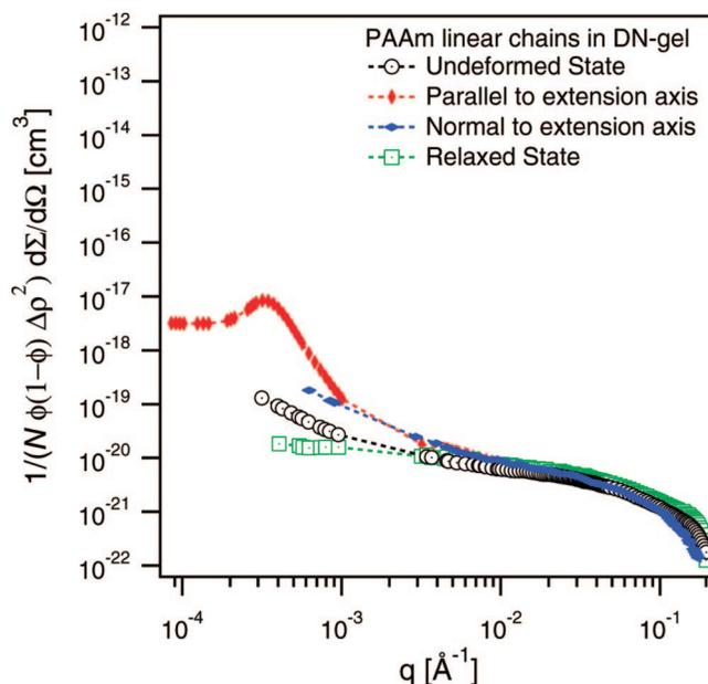
**Figure 2.** Neutron scattering from PAAm measured in situ for deformed DN gels (contrast condition i). Data parallel and normal to the elongation direction ( $y$  axis) are shown in red and blue, respectively. Results from the sample both before deformation (black) and after the deformation is relaxed (green) are also included for comparison. Markers are experimental data points, and dashed lines are drawn as a guide to the eye.
