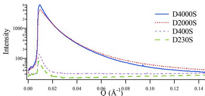
**Figure 3.** Small angle X-ray scattering from several networks created with the S epoxy and the Jeffamine diamines. Large-scale heterogeneities observed with the two longer Jeffamines (D4000S and D2000S), possibly due to cube aggregations, are not evidenced in the shorter tether networks. The statistical uncertainties in the intensity values are better than better than 20 %.
