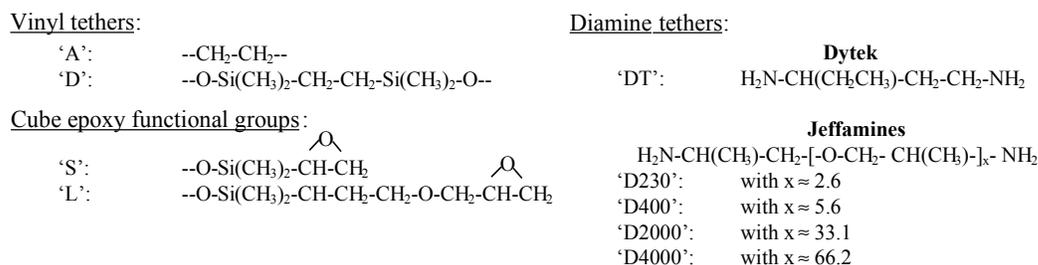
**Figure 1.** Molecular structures of the segments used in creating the organic tethers between the silsesquioxane cube. The nomenclatures to describe the segments are given in the quotations.
