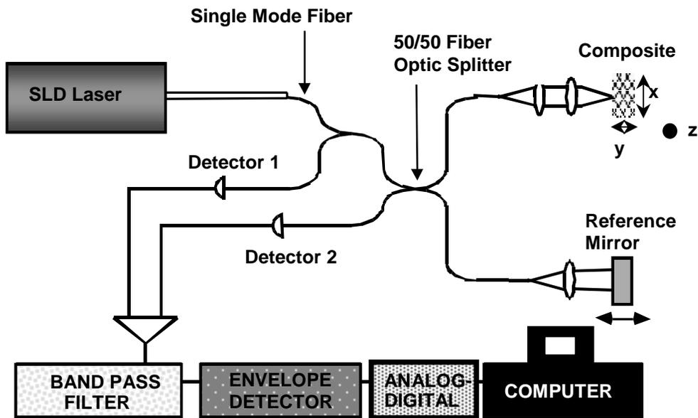
Figure 1: Schematic representation of the solid state laser and OCT system layout.
