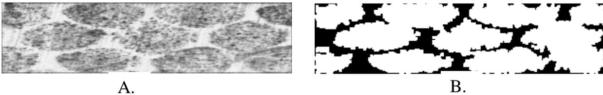
Figure 2: Original grayscale OCT image of the epoxy/ unidirectional E-glass composite. (A.), Binary OCT image after automated image processing (B.).
