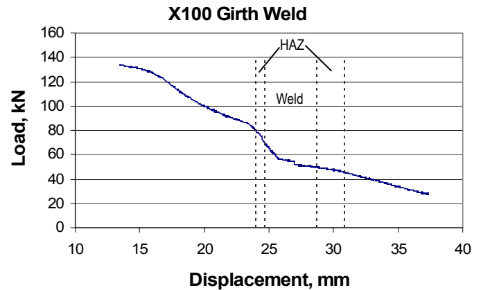
Figure 5. Typical load vs crosshead displacement plot across a girth weld. Note the load plateau in the weld, as the crack approaches the HAZ.
