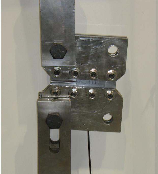
**Figure 2: A gripped specimen.**
