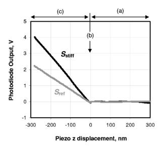
FIG. 2. Force-displacement curve examples (approach only) for a test cantilever contacting a stiff surface (bulk Si) and a reference cantilever
