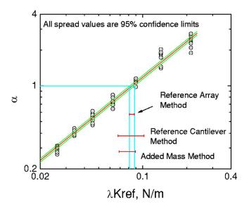
FIG. 4. (Color online) Reference cantilever array plot for a DNP-D test cantilever. Repeatabilities ( $\pm 2$  standard deviations) are compared to a single reference cantilever method and an added mass method.
