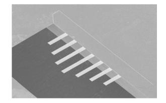
FIG. 3. Scanning electron micrograph of the experimental reference cantilever array. The cantilevers are nominally 1.4  $\mu$ m thick and 50  $\mu$ m wide and vary in length from 300 to 600  $\mu$ m.
