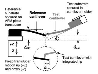
FIG. 1. Schematic diagram of the AFM configuration used for measuring the spring constant of an unknown test cantilever using a calibrated reference cantilever.
