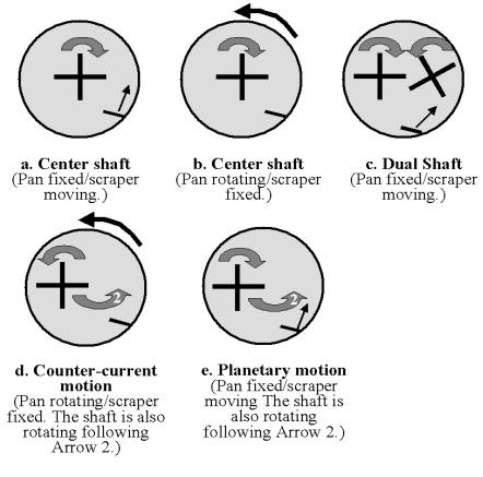
Fig 4. Various configurations for pan mixers. The arrows indicate the direction of rotation of the pan, blades, and scraper.
