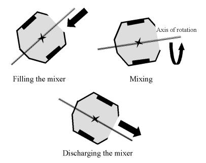
Fig. 3. Cross section of a tilting mixer.
