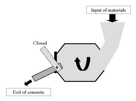
Fig. 2. Cross section of a non-tilting mixer [1].
