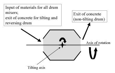
Fig. 1. Cross section of drum mixers.
