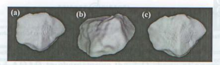
Fig. 3. (a) VRML visualization of Rock 1, (b) VRML visualization of Rock 2. The figure is not to scale, as Rock 2 is actually much smaller than Rock 1. (c) VRML visualization of Rock 1 based on numerical surface coordinates from X-ray CT.
