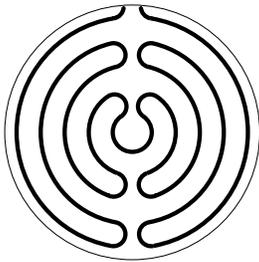
the layout of five circular heaters was transformed into a single heater, as shown in the inset, that reverses direction eight times, with the lengths of the reversing loops being the same as the lengths of the segments that are omitted, so that, while there will be small local perturbations in the temperature distributions near the reversing loops, the large-scale temperature distribution will be very similar to that for five circular heaters.
