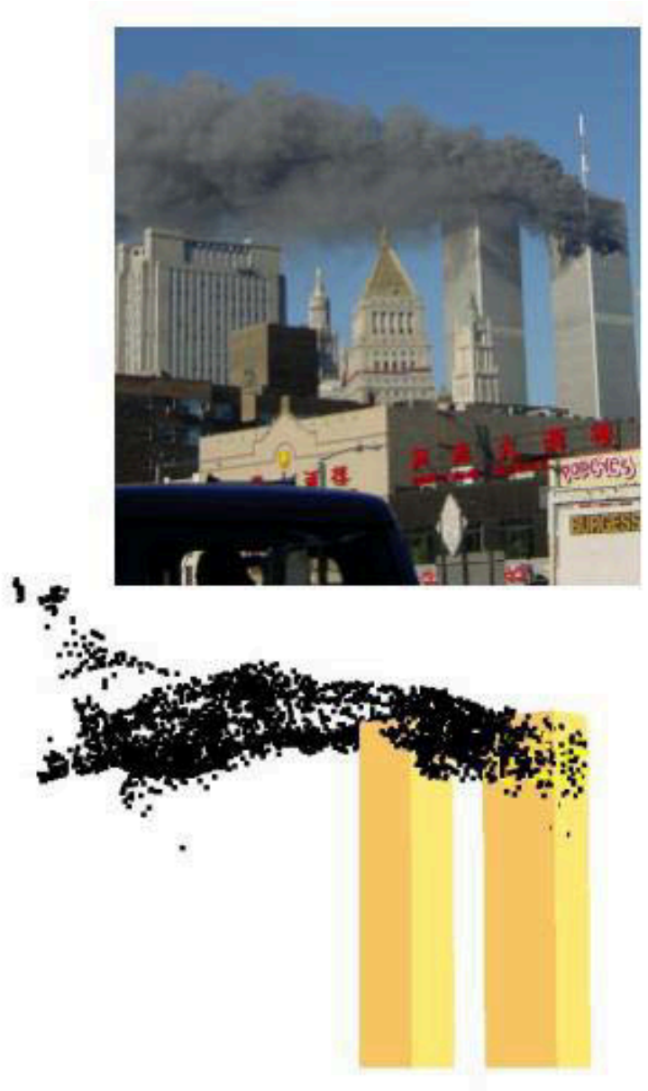
Figure 4: Comparison of a photograph ( ©2001 Kevin Ready. All rights reserved. Used by permission.) and of a frame from simulation of the WTC tower fires, showing the quasisteady smoke plume generated by the fire in the north tower.
