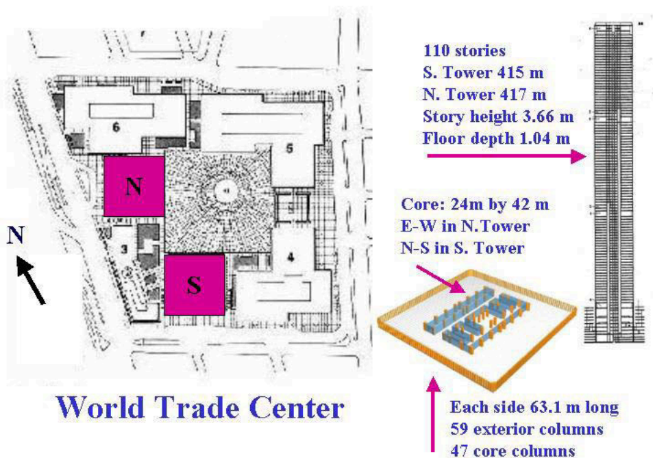
Figure 1: The layout of the World Trade Center complex and information about the twin towers. (WTC layout from web site www.greatbuildings.com . Floor layout from [8]. Vertical section of tower from [9].)
