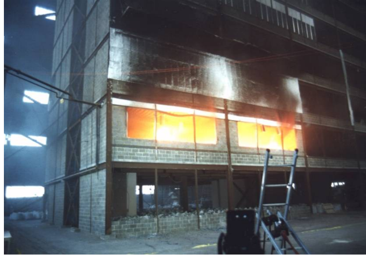
Figure 4. Full-scale steel structure built in Cardington Laboratory (left), and during a test fire (Usmani)
