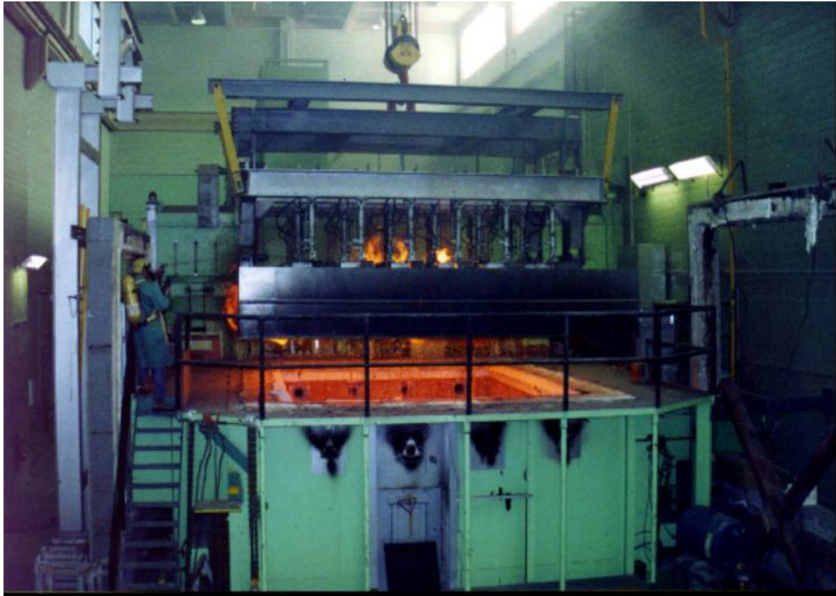
Figure 6. Photograph of modern floor testing furnace (Kodur)
