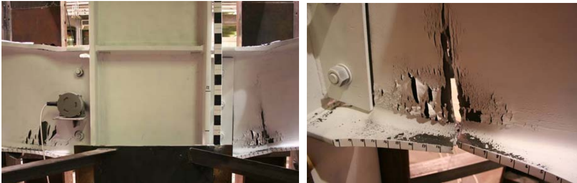
Figure 9: Failure mode of the RBS Test Specimen
