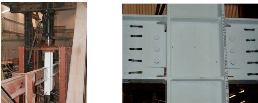
Figure 3: Photographs of the WUF-B Test Specimen
