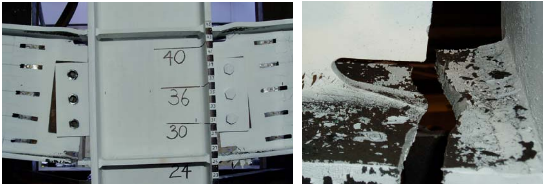
Figure 4: Failure mode of the WUF-B Test Specimen
