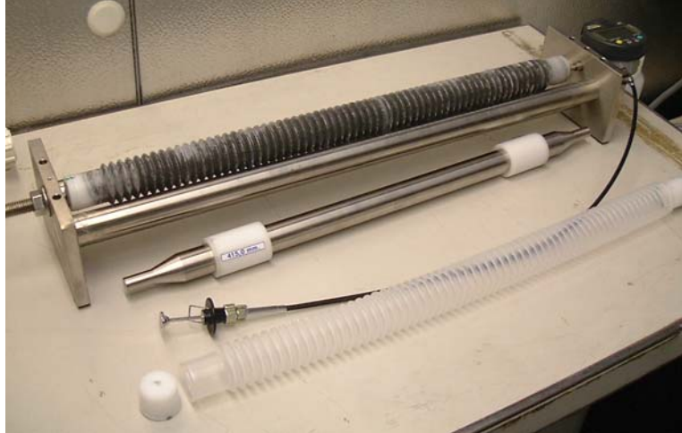
Figure 3. Typical equipment for measuring autogenous deformation of paste and mortar specimens. 4
