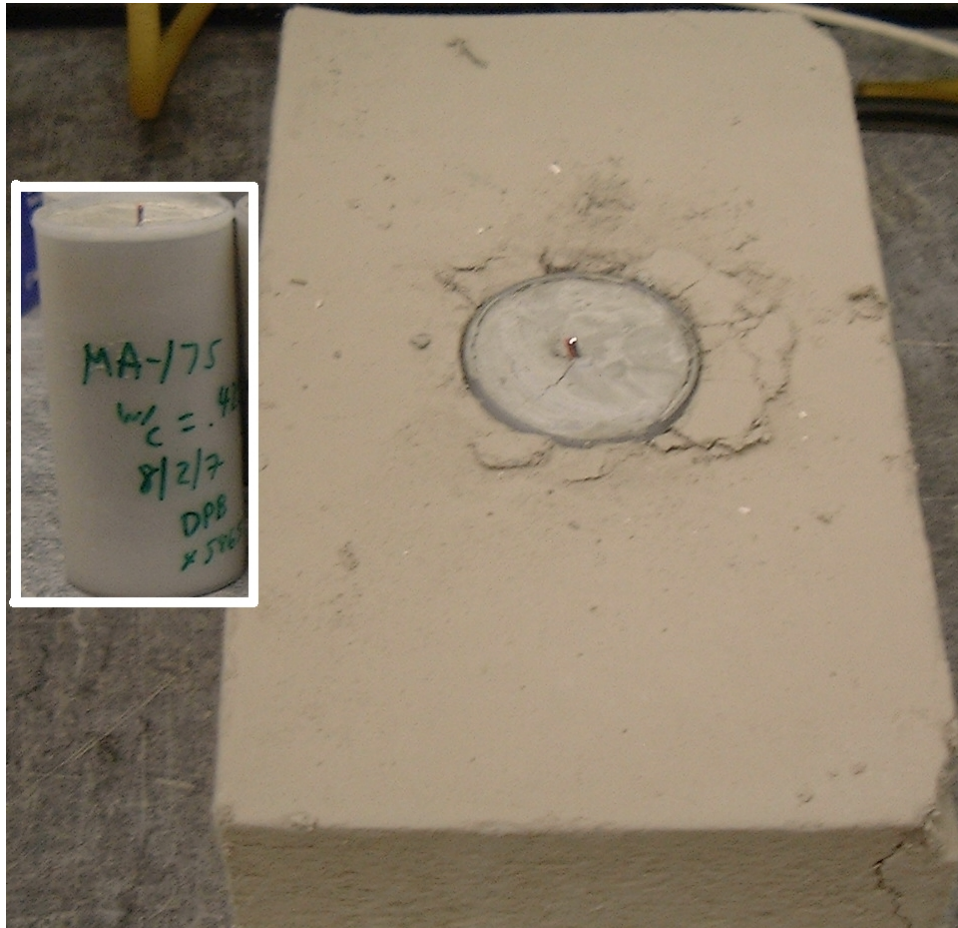
Figure 2. Custom-built semi-adiabatic calorimeter, with a typical size (48 mm diameter by 96 mm length cylinder) paste or mortar specimen (inset), embedded in microporous insulation. Top insulating panel is not shown.
