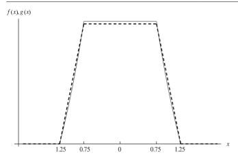
**Figure 5.** Comparison of the pdf f(x) of isocurvilinear trapezoidal distribution indicated by solid lines and the pdf g(x) of isosceles trapezoidal distribution indicated by dashed lines with the same parameters  $\mu - (\delta + \varepsilon)$ ,  $\mu - (\delta - \varepsilon)$ ,  $\mu + (\delta - \varepsilon)$  and  $\mu + (\delta + \varepsilon)$  for  $\mu = 0$ ,  $\delta = 1.0$  and  $\varepsilon = 0.25$ .
