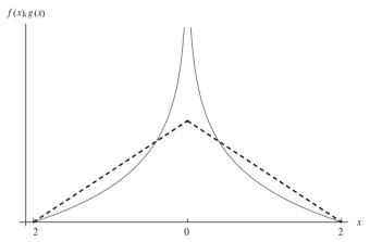
**Figure 8.** Comparison of the pdf f(x) of isocurvilinear trapezoidal distribution indicated by solid lines and the pdf g(x) of isosceles trapezoidal distribution indicated by dashed lines with the same parameters  $\mu - (\delta + \varepsilon)$ ,  $\mu - (\delta - \varepsilon)$ ,  $\mu + (\delta - \varepsilon)$  and  $\mu + (\delta + \varepsilon)$  for  $\mu = 0$ ,  $\delta = 1.0$  and  $\varepsilon$  tends to 1.0.
