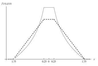
**Figure 7.** Comparison of the pdf f(x) of isocurvilinear trapezoidal distribution indicated by solid lines and the pdf g(x) of isosceles trapezoidal distribution indicated by dashed lines with the same parameters  $\mu - (\delta + \varepsilon)$ ,  $\mu - (\delta - \varepsilon)$ ,  $\mu + (\delta - \varepsilon)$  and  $\mu + (\delta + \varepsilon)$  for  $\mu = 0$ ,  $\delta = 1.0$  and  $\varepsilon = 0.75$ .
