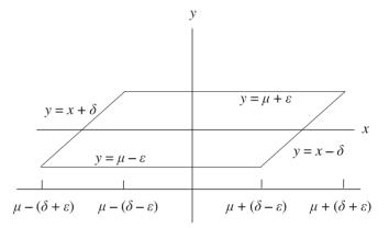
**Figure 2.** The region in the (x, y) plane where the joint pdf of  $X_S$  and *Y* has a positive value.
