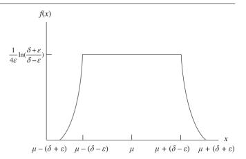
**Figure 3.** Probability density function f(x) of an isocurvilinear trapezoidal distribution with parameters  $\mu - (\delta + \varepsilon)$ ,  $\mu - (\delta - \varepsilon)$ ,  $\mu + (\delta - \varepsilon)$  and  $\mu + (\delta + \varepsilon)$ .
