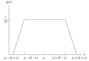
**Figure 1.** Probability density function g(x) of an isosceles trapezoidal distribution with parameters  $\mu - (\delta + \varepsilon)$ ,  $\mu - (\delta - \varepsilon)$ ,  $\mu + (\delta - \varepsilon)$  and  $\mu + (\delta + \varepsilon)$ .
