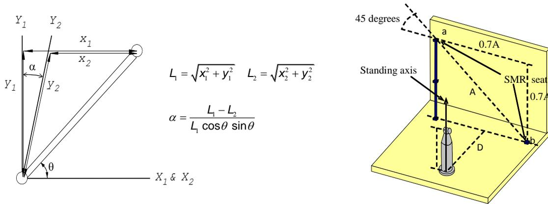
Figure 2: (left) diagram showing the effect of an axis squareness error; (right) one of the testing positions in the ASME B89.4.19 standard to detect this error source.
