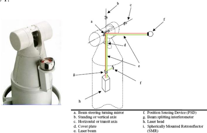
Figure 1: A schematic of the opto-mechanical construction of a laser tracker
