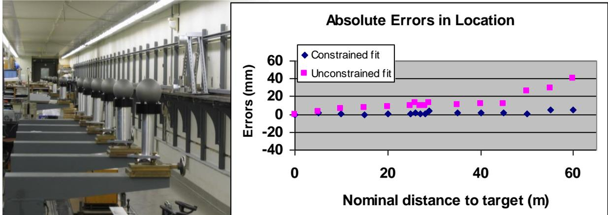
Figure 4: (left) A 1D test range spanning 66 meters using 101.6 mm diameter spheres as non-cooperative targets; (right) the absolute value of sphere center-to-center distance errors as a function of distance from the nearest sphere.
