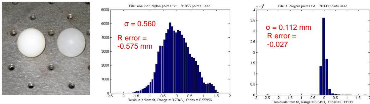
Figure 3: (left) photo of 25.4 mm nylon (L) and polypropylene (R) spheres; (middle) the fit residuals for the polypropylene sphere; (right) the fit residuals for the nylon sphere.
