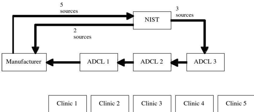
Figure 22-1. Transfer of NIST primary air-kerma-strength standard for brachytherapy sources to the ADCLs and manufacturer.
