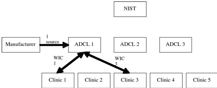
Figure 22-2. Calibration of clinical well-ionization chambers (WIC) by ADCL.
