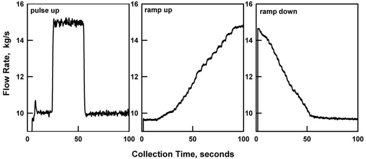
**Figure 6. Calculated flows based on time dependent dynamic mass flow model (Eq. 14) for three of the four unsteady flows studied in this work.**
