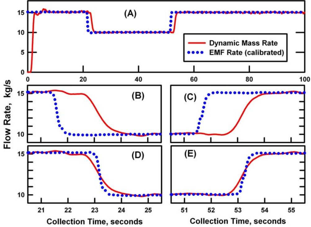
**Figure 5.** Flow deduced from the weigh scale data (dynamic mass rate) and from the electromagnetic flow meter. In panels (D) and (E), the EMF data are plotted 1.57 s after the recorded time.
