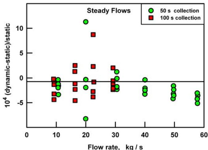
**Figure 3. Fractional differences between dynamic measurements and NIST's static gravimetric standard for steady flows from [2].**
