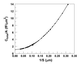
Fig. 3. Universal capacitance curve for chip C3B. Points are measured data, and the curve is the fit to data.
