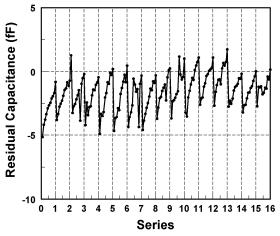
Fig. 4. Residual capacitance between devices with identical designs in different groups on the same chip. Each series consists of 11 devices.
