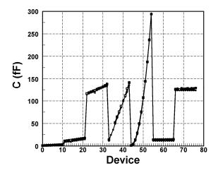
Fig. 5. Calculated and measured MIM capacitances versus device series. Theoretical data corrected for stray capacitance (solid circles) and measured capacitance for the two instruments (solid squares and open circles) are plotted.
