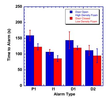
Figure 8. Average alarm time for flaming, polyester fabric, bedroom fires. Comparison between configuration 8 (door open, high density foam) and configuration 6 (door closed, low density foam. Error bars are one standard deviation.
