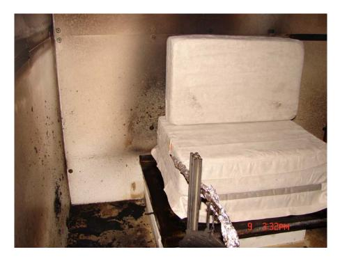
Photo 1. Flaming ignition of a chair mockup. The ignitor was removed after 40 s.
