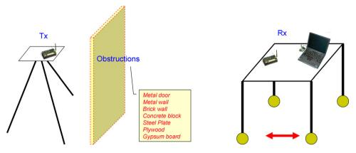
Fig. 1. Schematic of test setup.
