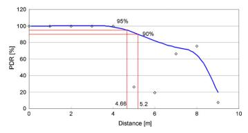
Fig. 7. PDR vs. distance for transmission in an open field at -25 dBm.
