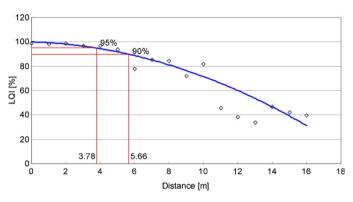
Fig. 9. LQI vs. distance for transmission through brick wall at 0 dBm.
