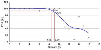
Fig. 10. PDR vs. distance for transmission through brick wall at 0 dBm.
