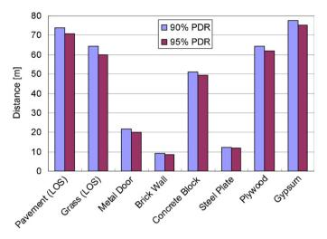
Fig. 14. Maximum separation distances between transmitters operating at 0 dBm and receivers to attain packet delivery rates of 90% and 95%.
