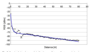
Fig. 2. Received signal strength indication vs. distance for transmission in an open field at 0 dBm.
