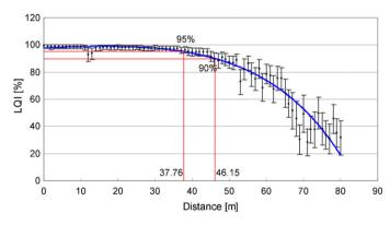
Fig. 3. Link quality indication vs. distance for transmission in an open field at 0 dBm.
