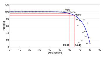
Fig. 4. Packet delivery rate vs. distance for transmission in an open field at 0 dBm.
