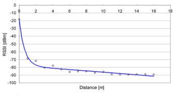
Fig. 8. RSSI vs. distance for transmission through brick wall at 0 dBm.
