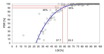
Fig. 12. Packet delivery rate vs. link quality indication for transmission in an open field at 0 dBm and no obstructions.
