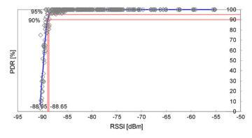
**Fig. 11.** Packet delivery rate vs. RSSI for transmission in an open field at 0 dBm and no obstructions.
