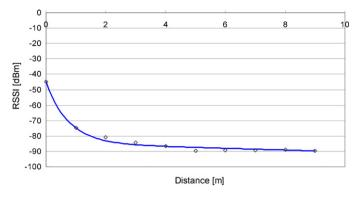
Fig. 5. RSSI vs. distance for transmission in an open field at -25 dBm.
