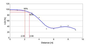
Fig. 6. LQI vs. distance for transmission in an open field at -25 dBm.
