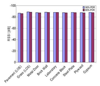
Fig. 13. RSSI at 90% and 95% PDR's for different materials, signals transmitted at 0 dBm.
