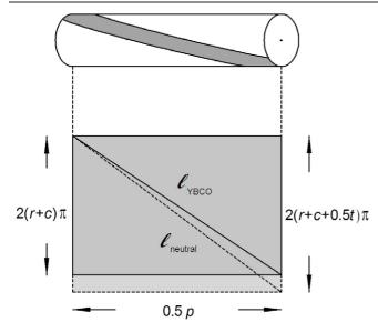
**Figure 3.** Schematic of the different path lengths between the YBCO layer and the neutral axis of a coated conductor that is wound around a former with twist pitch *p*.
