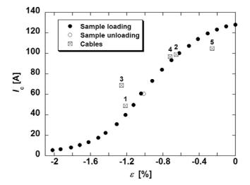
**Figure 1.** Critical current as a function of axial compressive strain at 76 K of a YBCO coated conductor that is soldered on a brass bending beam. The applied strain is measured directly on the surface of the sample with a strain gage. The critical currents at the calculated strain state of prototype cables (numbered) are included (below, table 1).
