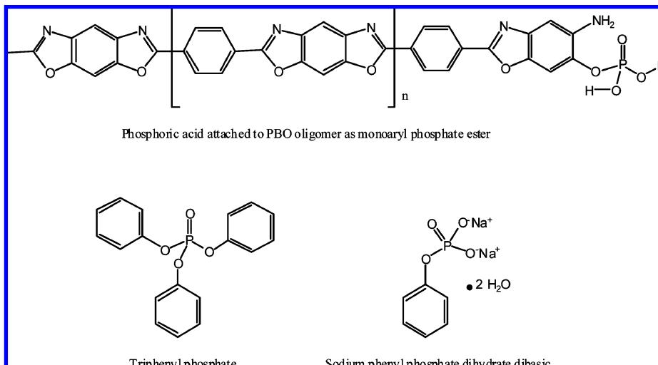
**Figure 5.** Chemical structure representation of phosphoric acid chemically bound to PBO oligomer as a monoaryl phosphate ester. To underscore the stability of the monoaryl phosphate ester bond, the chemical structures of triphenyl phosphate (a triaryl phosphate ester) and sodium phenyl phosphate dibasic (a monoaryl phosphate ester), which are available commercially, are also shown.
