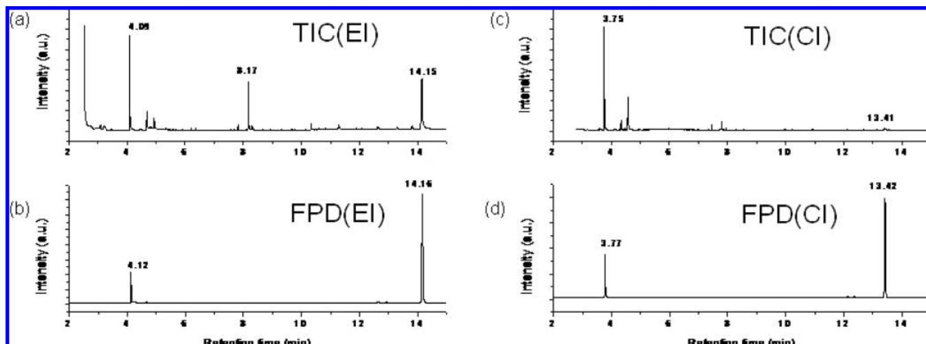
**Figure 3.** Total ion current (TIC) chromatograms (a) and (c) and parallel flame photometric detector (FPD) chromatograms (b, d) of methylated aqueous extract from PBO fibers under electron impact (EI) (a, b) and chemical ionization (CI) (c, d) test conditions. A.U. denotes arbitrary units of intensity.
