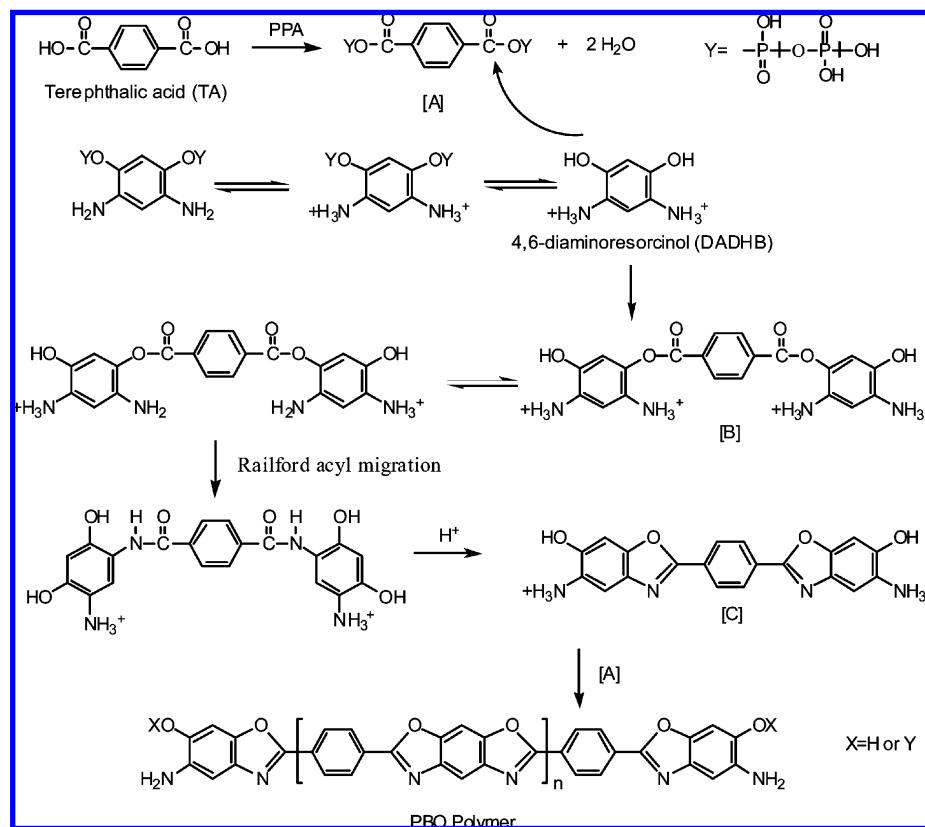
**Figure 1.** Reaction scheme for the preparation of PBO polymer (adapted from ref 6 1997 American Chemical Society and ref 7 1998 American Chemical Society).
