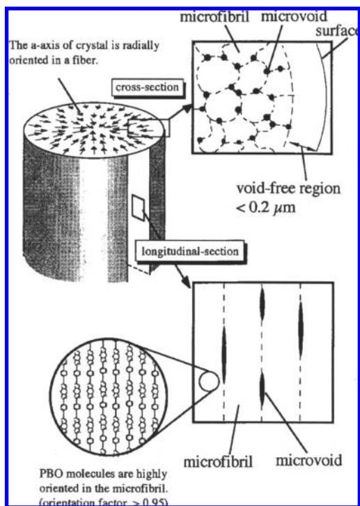
**Figure 2.** PBO structure model of AS fiber. (Reprinted with permission from ref 15. Copyright 1998 Wiley).
