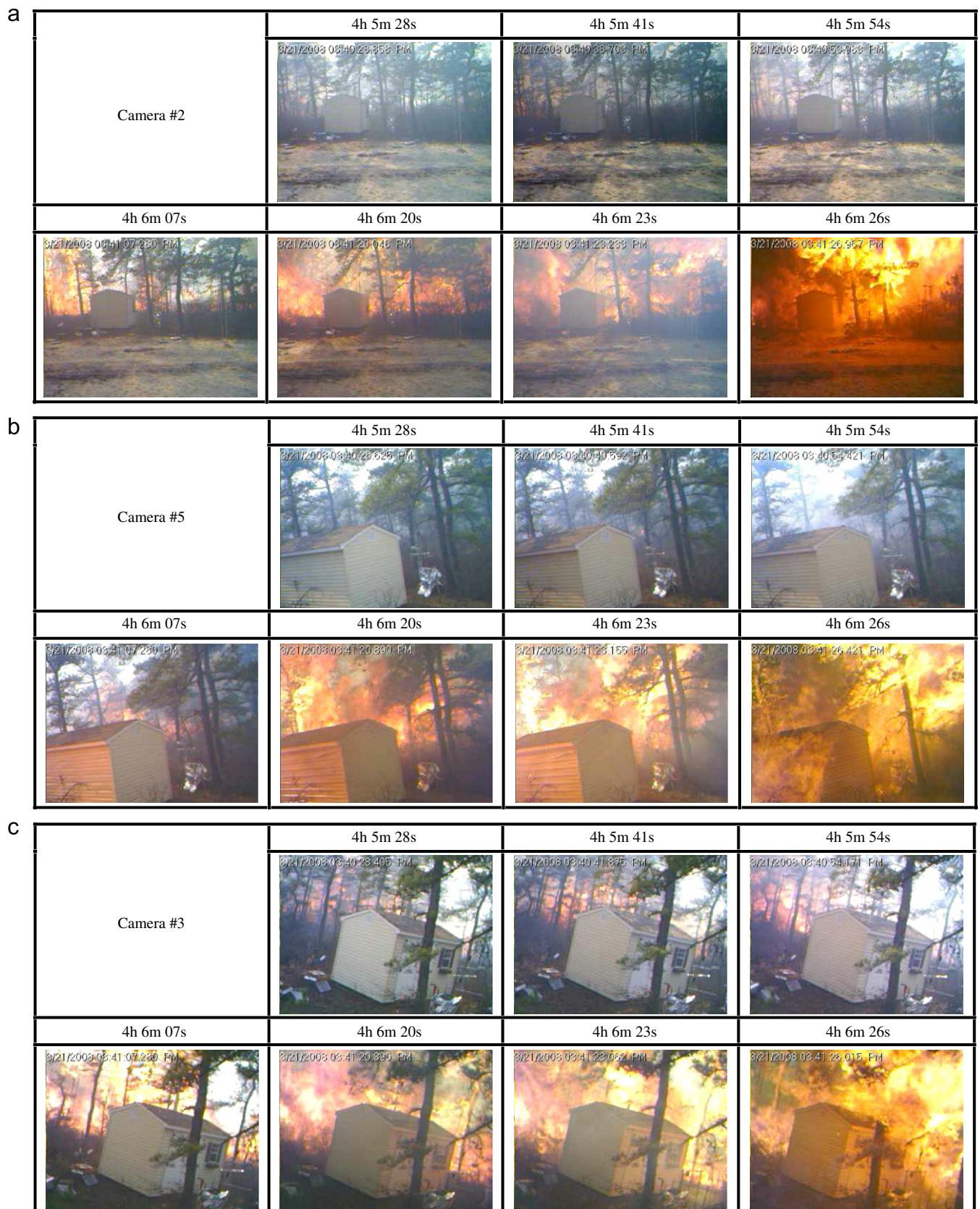
Fig. 6. (a)–(c) In-situ temporally resolved images of fire front spread; the data loggers and cameras were started approximately four hours before the fire was ignited.
