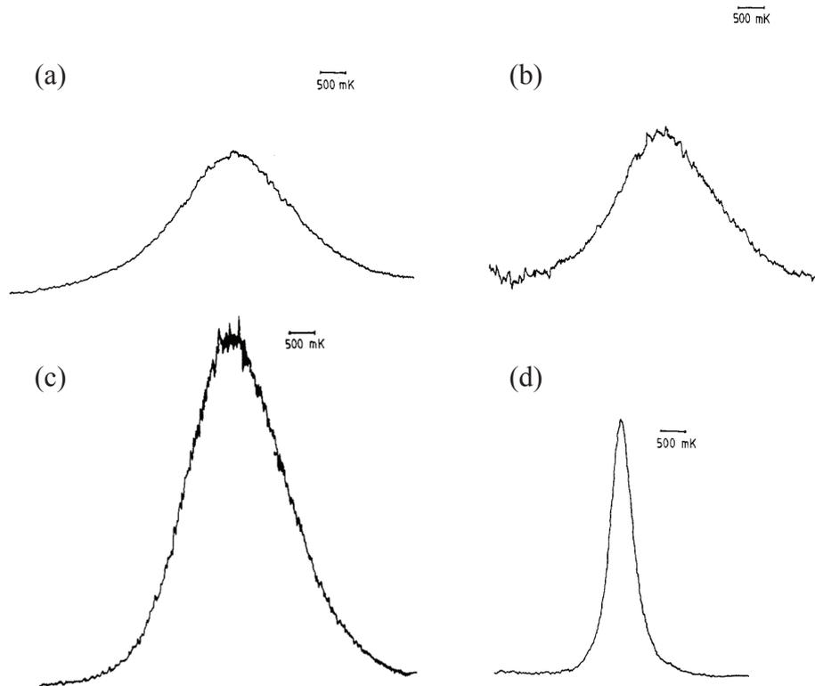
FIG. 4 Optogalvanic spectra of Cd I autoionizing resonances: (a)  $5s5p\ ^3P_2-5p^2\ ^3P_1$  at 232.9 nm, (b)  $5s5p\ ^3P_1-5p^2\ ^3P_1$  at 226.7 nm, (c)  $5s5p\ ^3P_0-5p^2\ ^3P_1$  at 224.0 nm, (d)  $5s5p\ ^3P_1-5p^2\ ^3P_0$  at 230.7 nm. Inverse wavelength on the horizontal scale measured in  $\text{K}=\text{cm}^{-1}$ . [Reprinted figures with permission from Aymar *et al.* (1986). Copyright 2002 Institute of Physics.]
