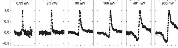
FIG. 8 Absorption profiles for single quantum dot spectroscopy (Kroner *et al.*, 2008), at increasing value of the laser power, from 0.33 nW on the far left up to 22 nW on the far right. Symbols represent the experimental data and solid lines are a guide to the eye based on the Fano lineshape. [Reprinted figure with permission from Kroner *et al.* (2008). Copyright 2008 of Nature.]
