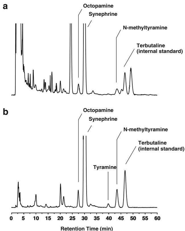
**Fig. 3** Separation of SRM 3258 with **a** absorbance detection at 220 nm (method 1) and **b** fluorescence detection (excitation 273 nm, emission 304 nm; method 2)
