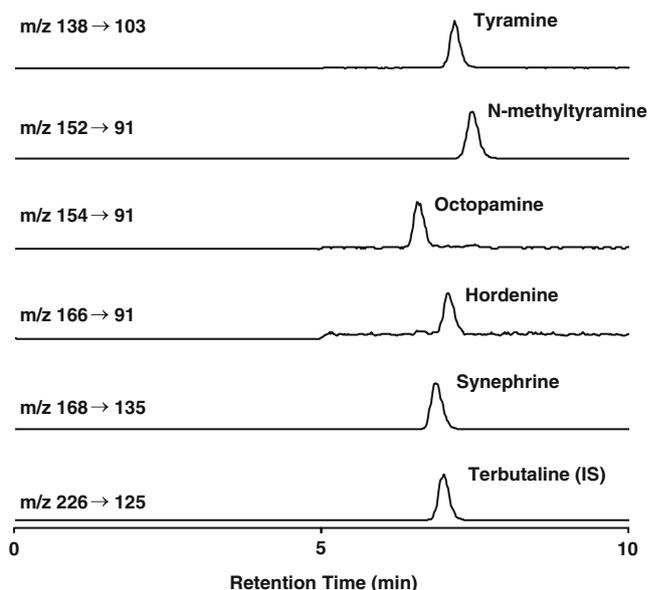
**Fig. 5** Representative multiple reaction monitoring chromatograms from the LC/MS/MS analysis of SRM 3259
