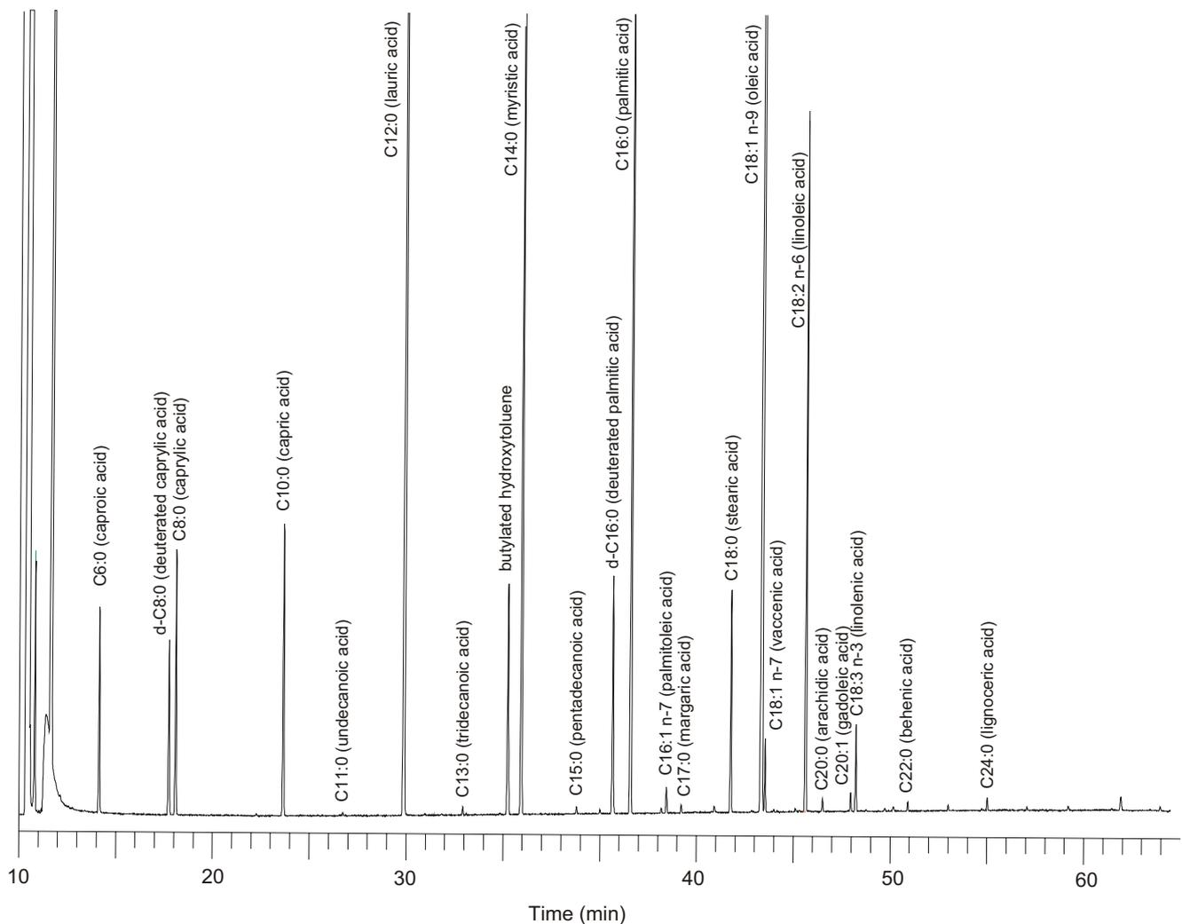
**Fig. 3** Typical chromatogram for the measurement of fatty acids in SRM 3251 using GC-FID on a nonbonded biscyanopropyl polysiloxane column. The column was held isothermally at 100 °C for 4 min and then temperature programmed at 2.5 °C/min to 240 °C where it was held
